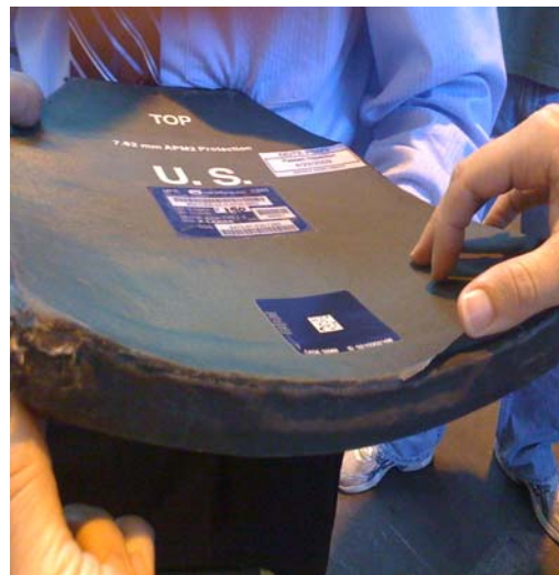
Figure 22. ESAPI at Fort Lewis with a Passed Inspection Label and an External Material Failure
