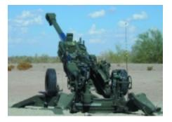
of less than 9,800 pounds (with digital fire control). It offers greater ground mobility and improved reaction times compared to the M198 howitzer it is designed to replace.
