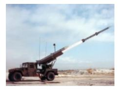
with the Advanced Medium Range Air-to-Air Missile (AMRAAM) on a HMMWV platform, missile interface equipment, remote terminal units, a three-axis geographic position system, a GPS receiver, SINCGARS radios, and a reloading device.
