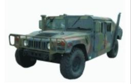
include a 15-year corrosion prevention package, fully independent suspension, electronically controlled, four-speed automatic transmission, an EPA-compliant 6.5L diesel engine, improved brakes, an improved electrical system, three-point seatbelts, and increased payload capacity.
