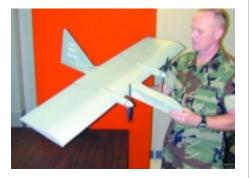
The Dragon Eye air vehicle is the key component of SURSS. Dragon Eye is a five-pound UAV that flies at 35 knots at altitudes of 300-500 feet above the ground. The vehicle, which is hand-launched by two Marines, flies a preprogrammed route using Global Positioning Satellite waypoints to navigate. Once in the area of interest it uses on-board sensors to gather and transmit imagery back to the ground control station. The system is man-portable, and can be recovered and reused.
