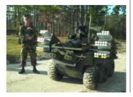
operations. The primary function of the Gladiator will be to provide the Ground Combat Element with unmanned scouting and reconnaissance, surveillance, and target acquisition.
