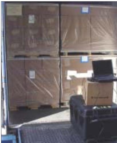
(Above) A portable reader determines the ability to read Type 3 tags on pallets already loaded into a container during preliminary testing at Defense Distribution Depot San Joaquin. (Top right) Type 1 case tags are read while simulating loading and unloading through an entrance and exit portal. (Bottom right) A flatbed truck drives past a reader scanning Type 3 pallet and container tags. Courtesy photos
