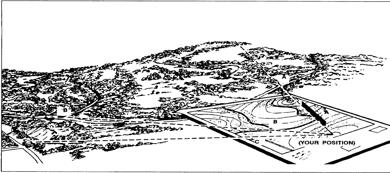
Figure 6-19. Resection with straightedge.
