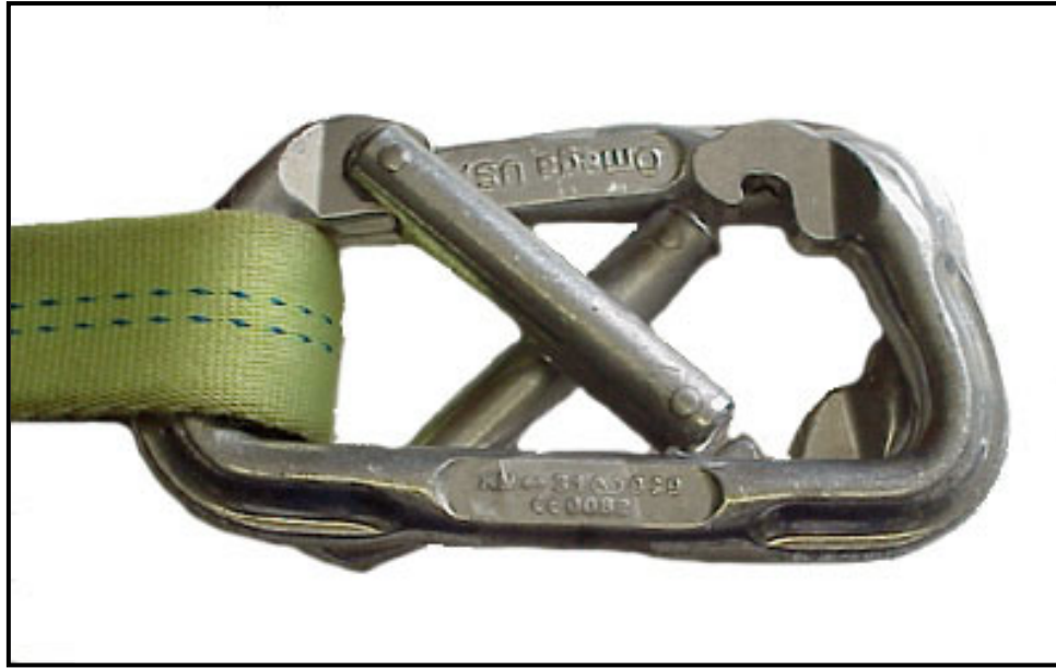
Figure 5-6. Correctly opposed carabiners.
