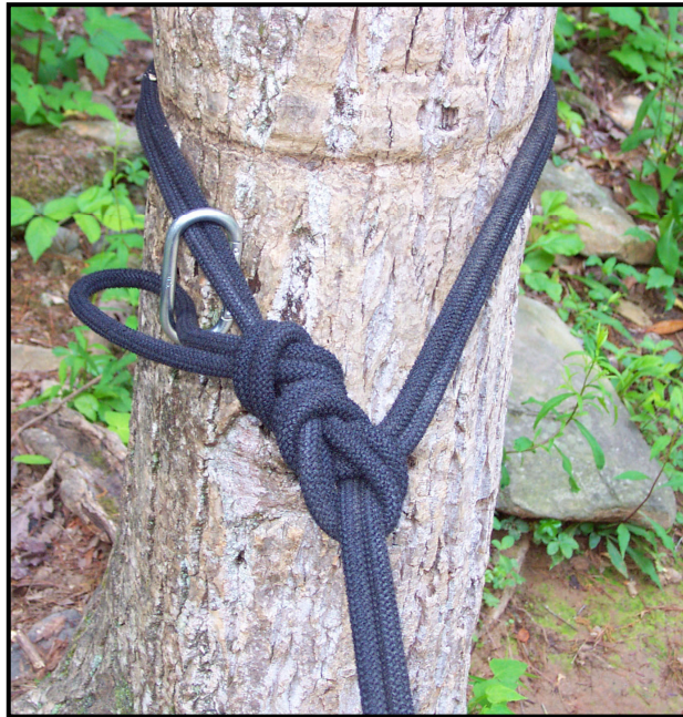
Figure 5-10. Rope tied to anchor with anchor knot.
