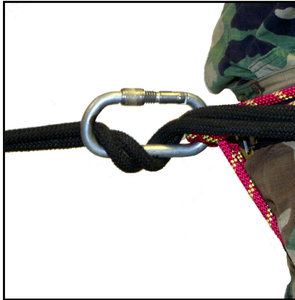
Figure 7-7. Proper hookup using carabiner wrap.
