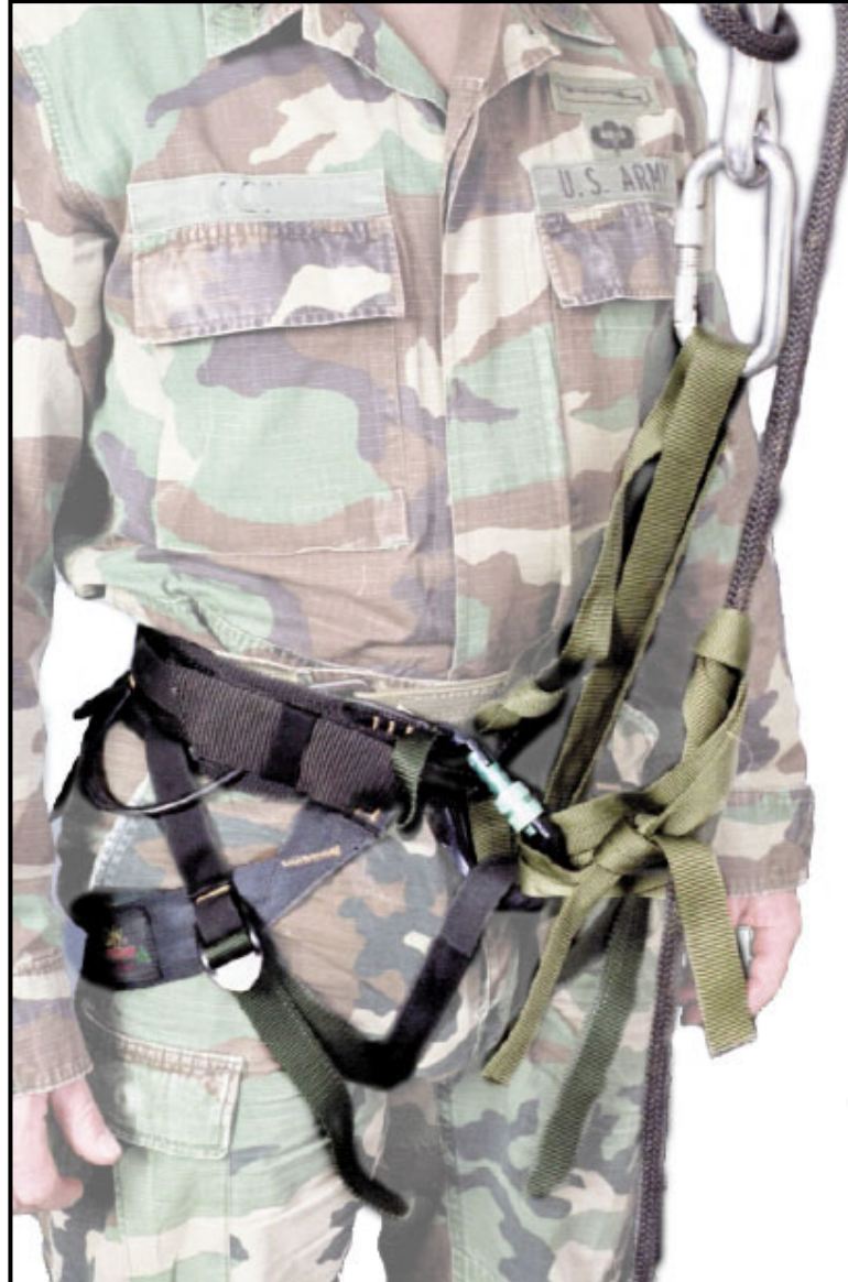
Figure 7-9. Extended hookup with self-belay.
