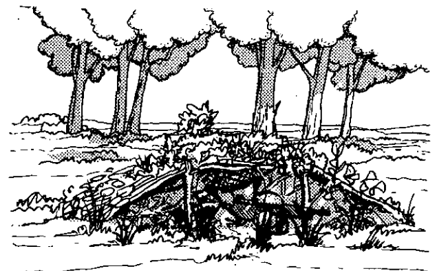
① FOXHOLE WITH CAMOUFLAGE COVER IN PLACE
