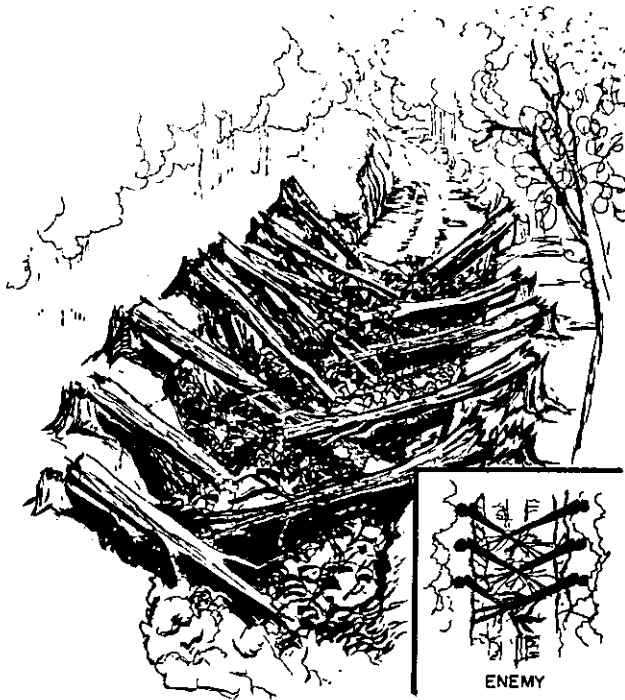
Figure 7-8. Abatis used as roadblock.
