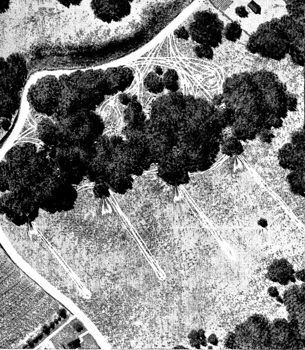
FIGURE 64 ①.—An artillery position can be simulated perfectly without the use of dummy guns or equipment. This decoy consists of blast marks, tracks, and debris.
