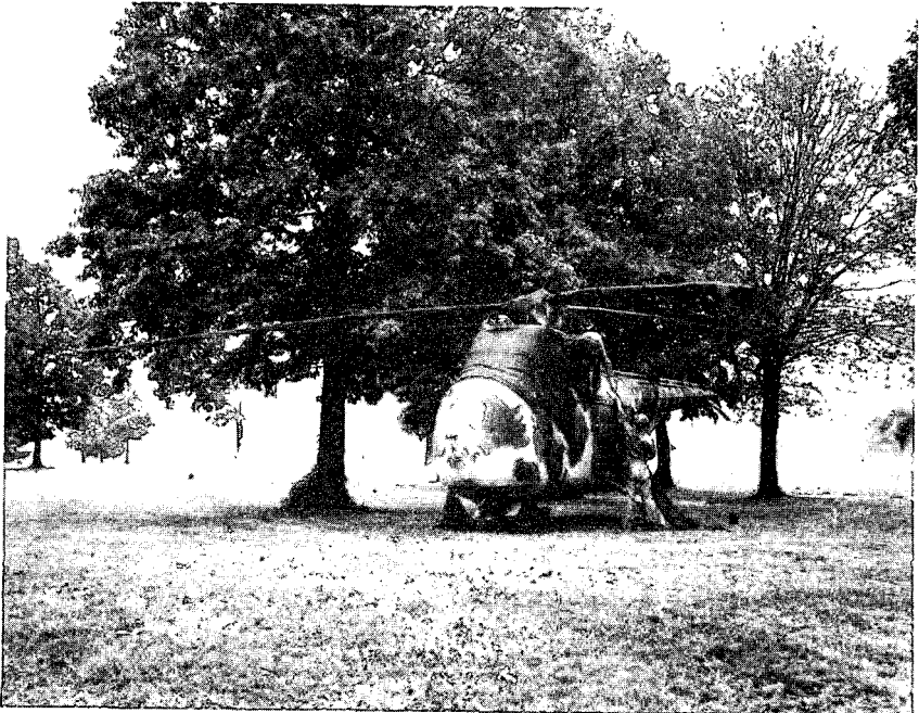
Figure 194. Covering shine and insignia on H-19 helicopter.
