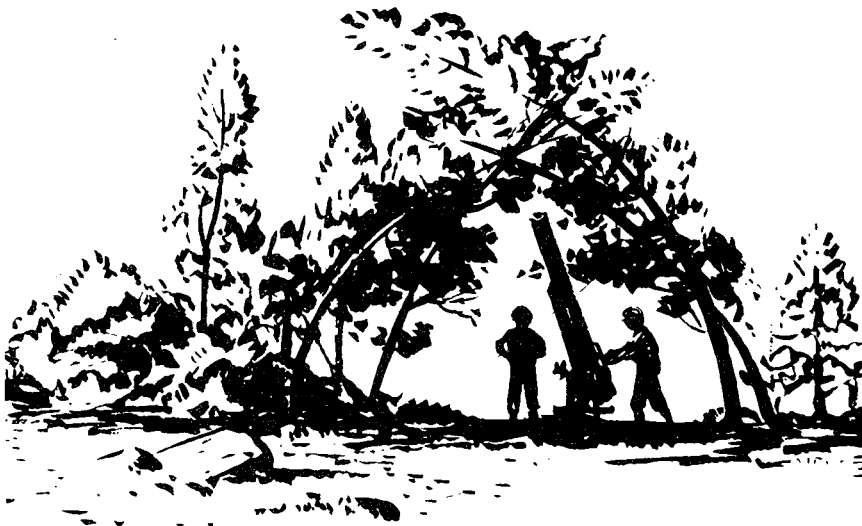
Figure 147. Small trees bent to conceal exposed area.
