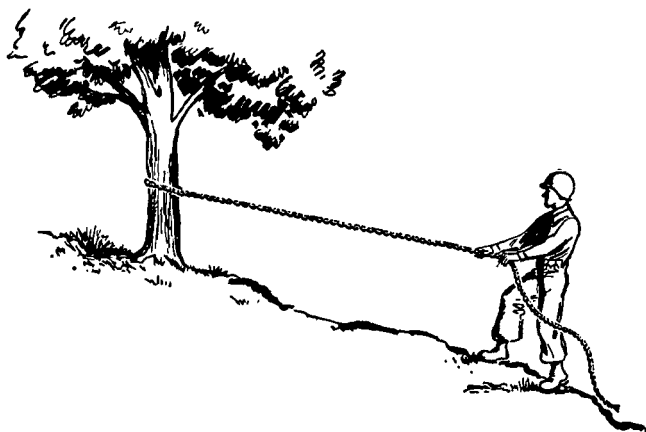
Figure 42. Simple fixed rope.
