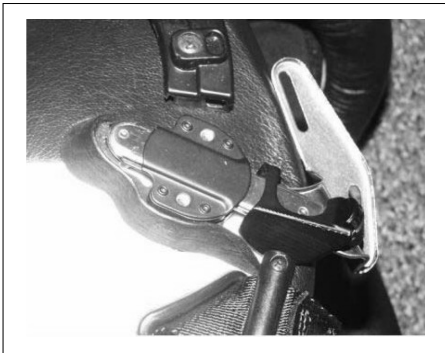
Figure 3-16. “New-Style” Bayonet Fittings
