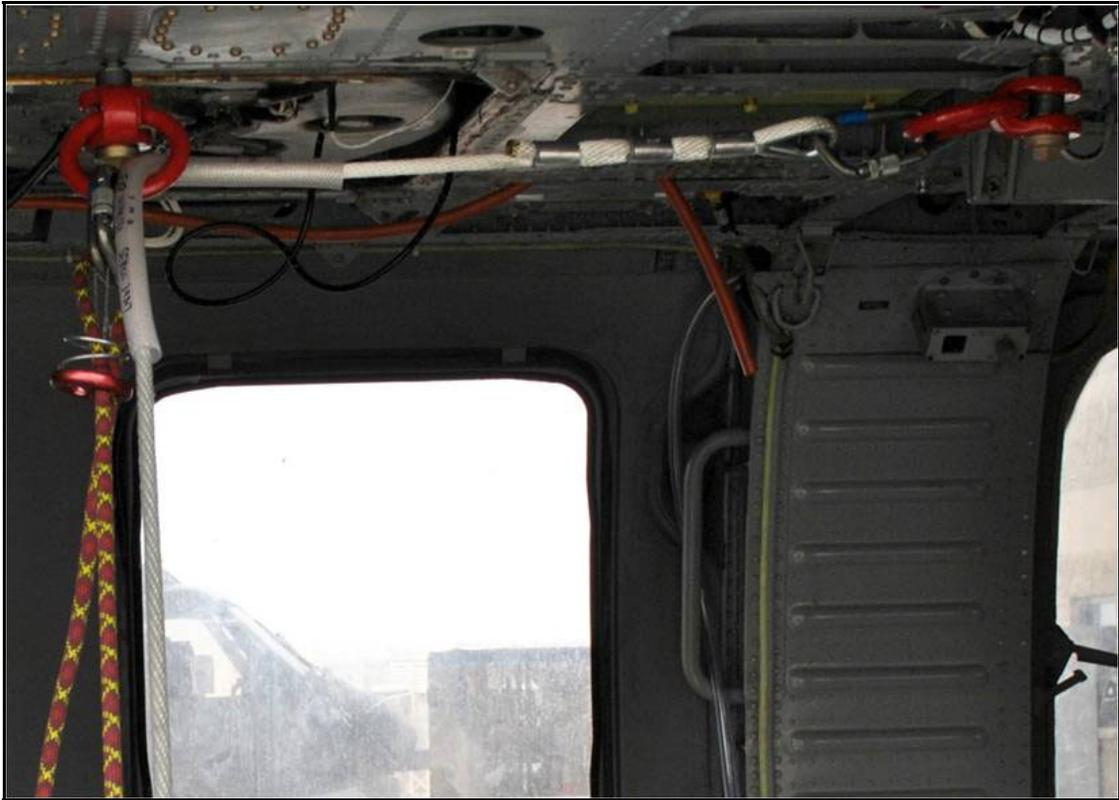
Figure 4-15. H-60 Red Rappel Rings Belay Set-Up
