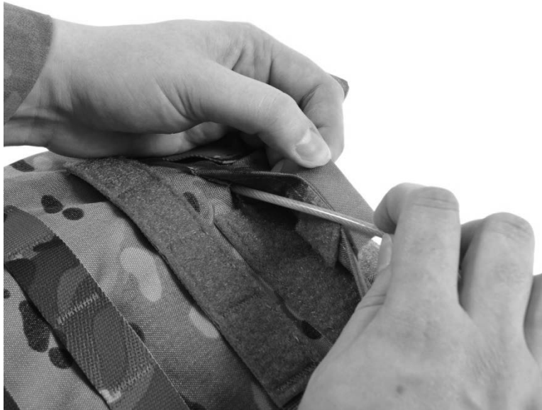
Figure 40. Cable Ends through Holes in Cable Release Pocket.
