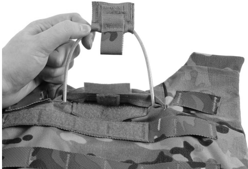
Figure 41. Pulling Both Cables through Holes.
