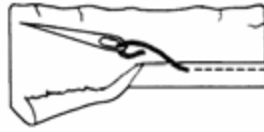
Figure 3. Turn Edge Under and Sew.
