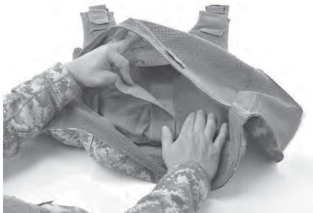
Figure 7. Re-sealing the Hard Armor Protective Insert Pocket.
