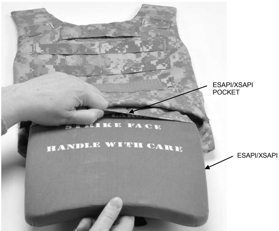
Figure 38. Removing ESAPI/XSAPI from Pocket.
