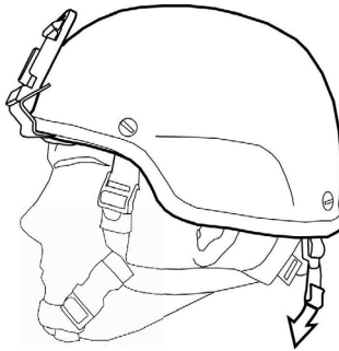
Figure 4. Tighten Rear Adjustment Straps (Universal H-Back Retention Systems).
