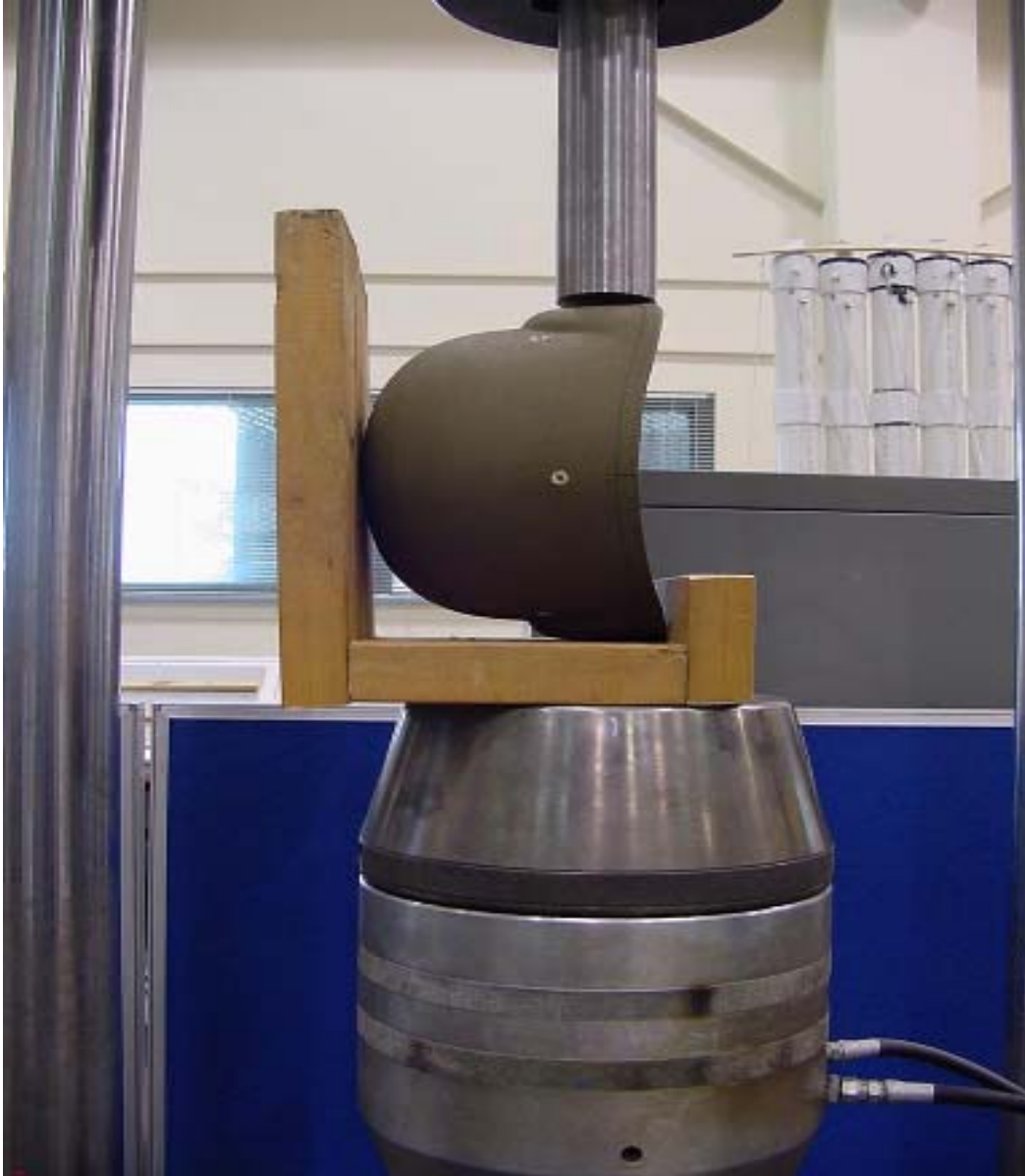
FIGURE 5. Jig for side to side compression resistance.
