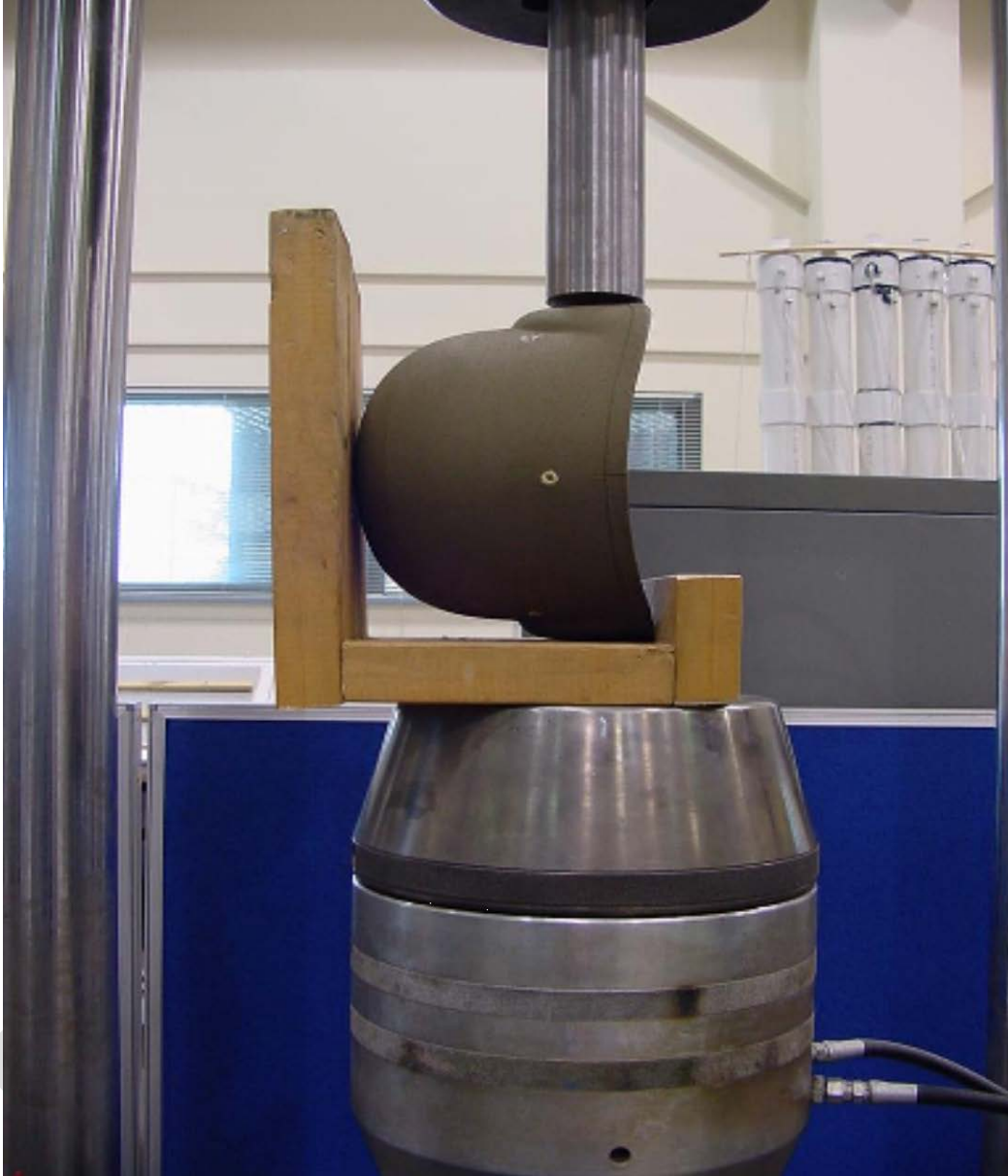
Figure 5. Jig – Side to Side Compression Resistance.
