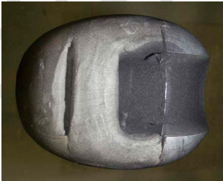
PICTURE 2. Headform: Rear Pad Support for Ballistic Hardware Testing
