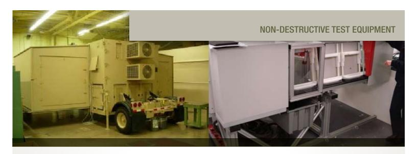
Non-Destructive Test Equipment (NDTE) uses digital X-rays to detect any physical or structural defects in body armor plates, and thus to ensure that Soldiers are equipped with mission-capable body armor while in theater. NDTE is a portable, deployable, self-contained system that can scan a plate in 15 seconds or less, or as many as 240 in an hour.
