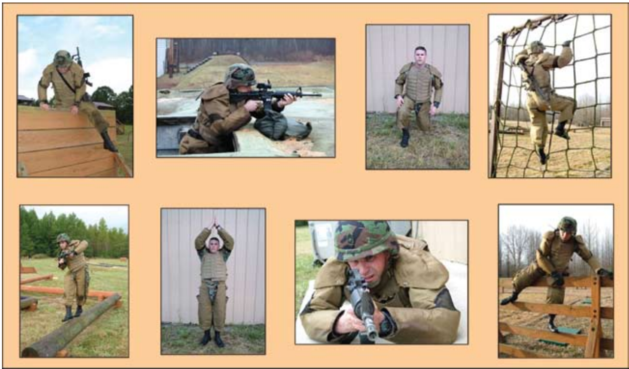
FIGURE 3 QuadGard testing by Army Research Laboratory at Aberdeen Test Center obstacle course and marksmanship range demonstrates the flexibility of the design and its compatibility with existing body armor and infantry equipment.
