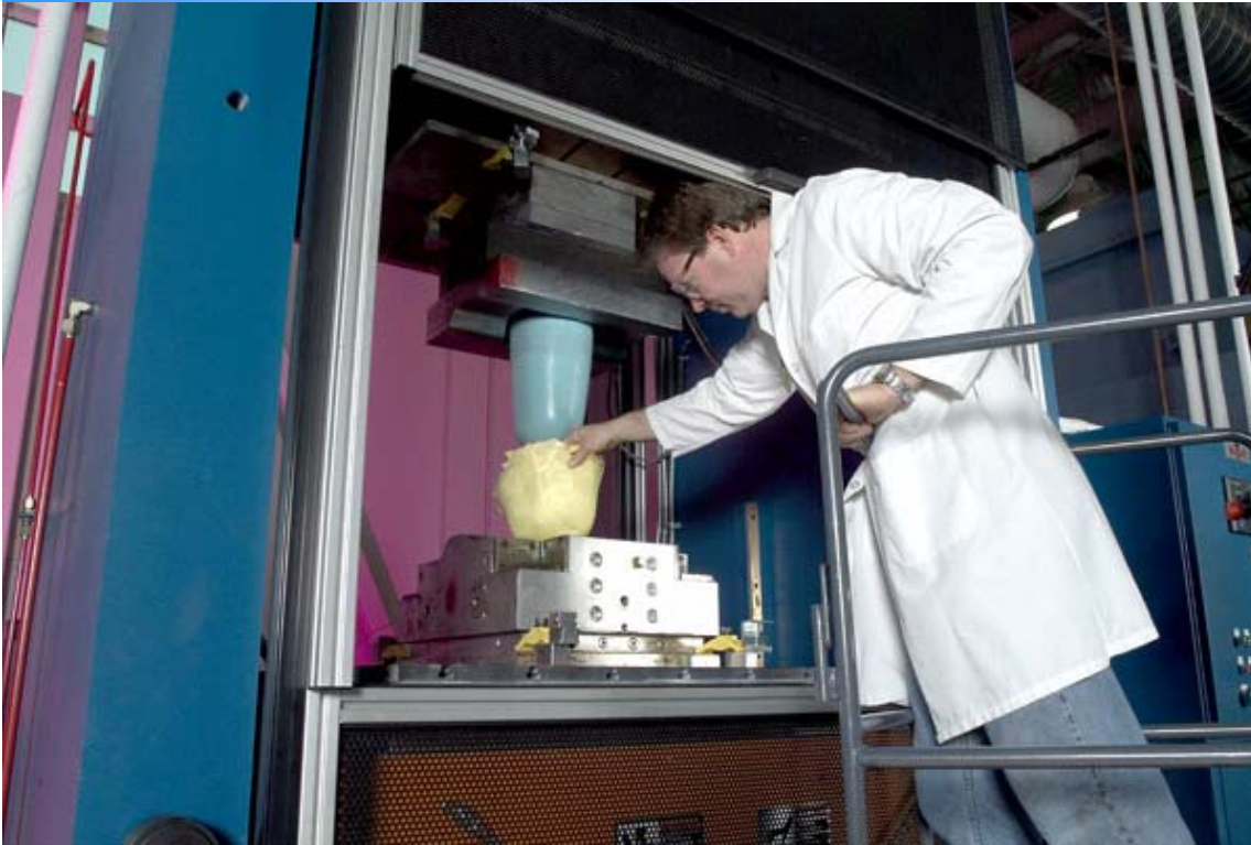
INSTALLATION OF TOOL & MATERIAL IN HYDRAULIC PRESS
