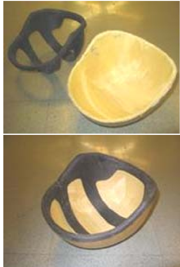
Fig. 11. Integrated helmet stiffener and suspension concept
