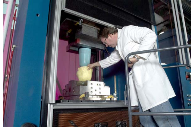
Fig. 6. Silicon plug, metal female cavity, thermoplastic preform placement
