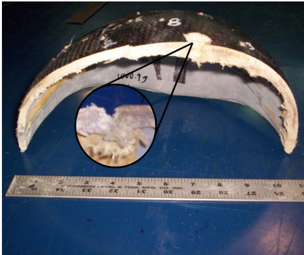
Fig. 10. Sectioned helmet with details of V50 testing
