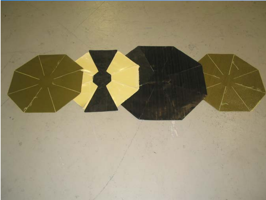
HYBRIDIZED MATERIALS (KEVLAR, GRAPHITE FIBER)
