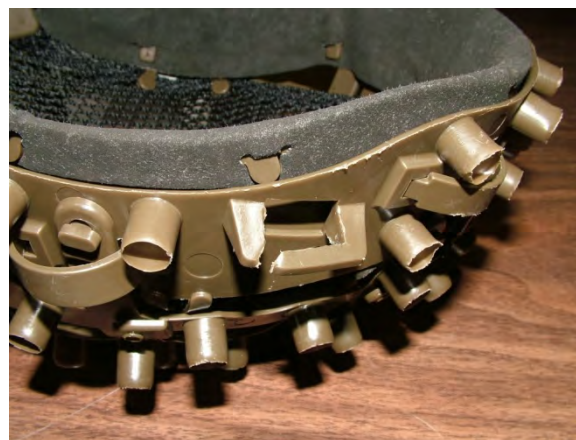
Figure 23. Suspension system “B” (note the broken mounting tab).
