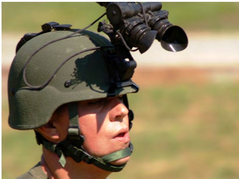
Figure 19. Forward rotation of the LWH with “A” and mounted NVG as the participant maneuvered on the obstacle and IMT courses.
