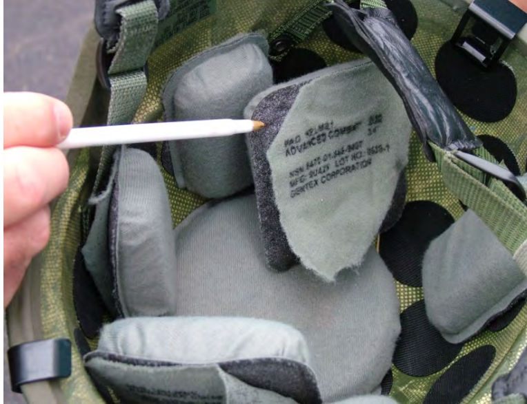
Figure 18. Helmet “A” suspension pads after the pads were removed from the helmet to wash. (Some of the hook and loop fastener dots were pulled away from the interior of the helmet.)
