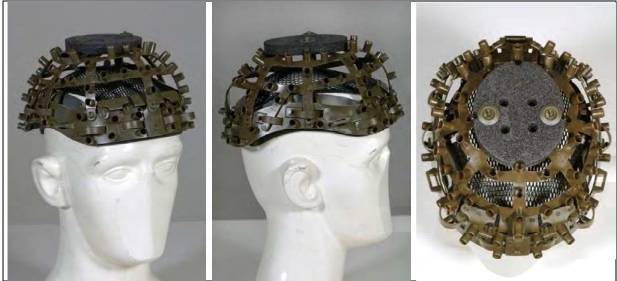
Figure 2. Views of the HeadGard or “B” suspension system (note the two helmet retention loops in photograph to the right).
