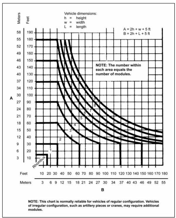
Figure C-2. Module determination chart
