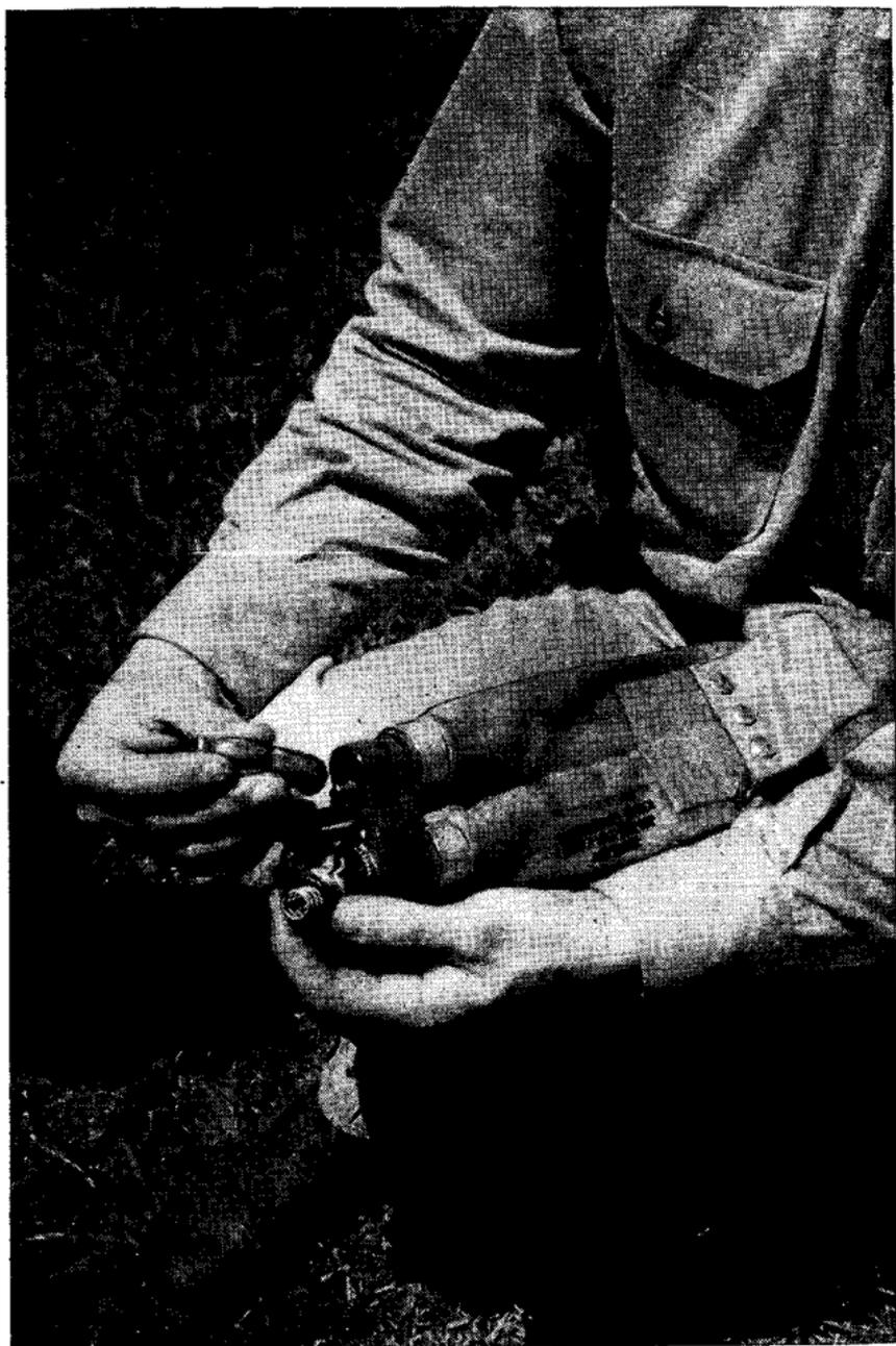
*Figure 9. Inserting carbon dioxide cartridges into life belt.*
