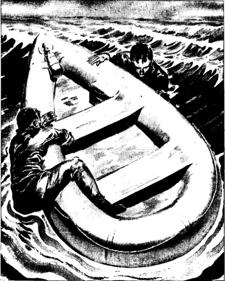
*Figure 21. Method of boarding rubber boat.*
