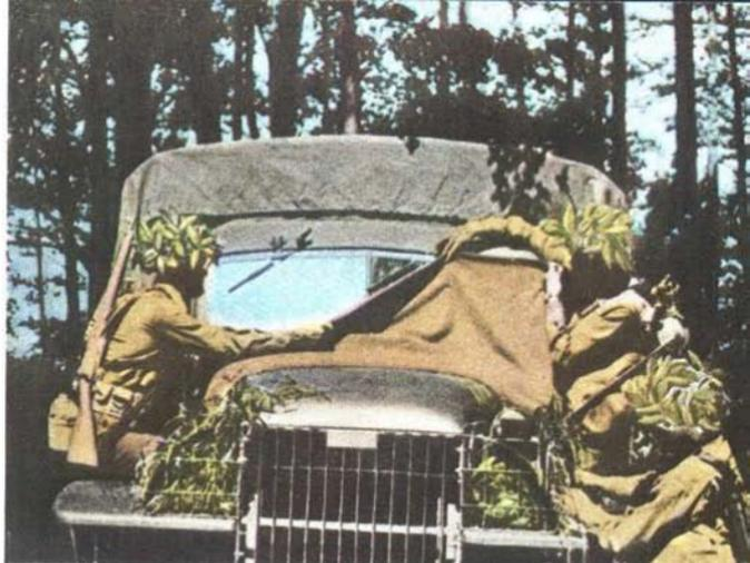
FIGURE 21. — The wise driver makes his own slip-on covers for headlights, windshields, and other reflecting surfaces. He keeps them covered at all times, if possible. They may be made of burlap, osnaburg, or salvage.
