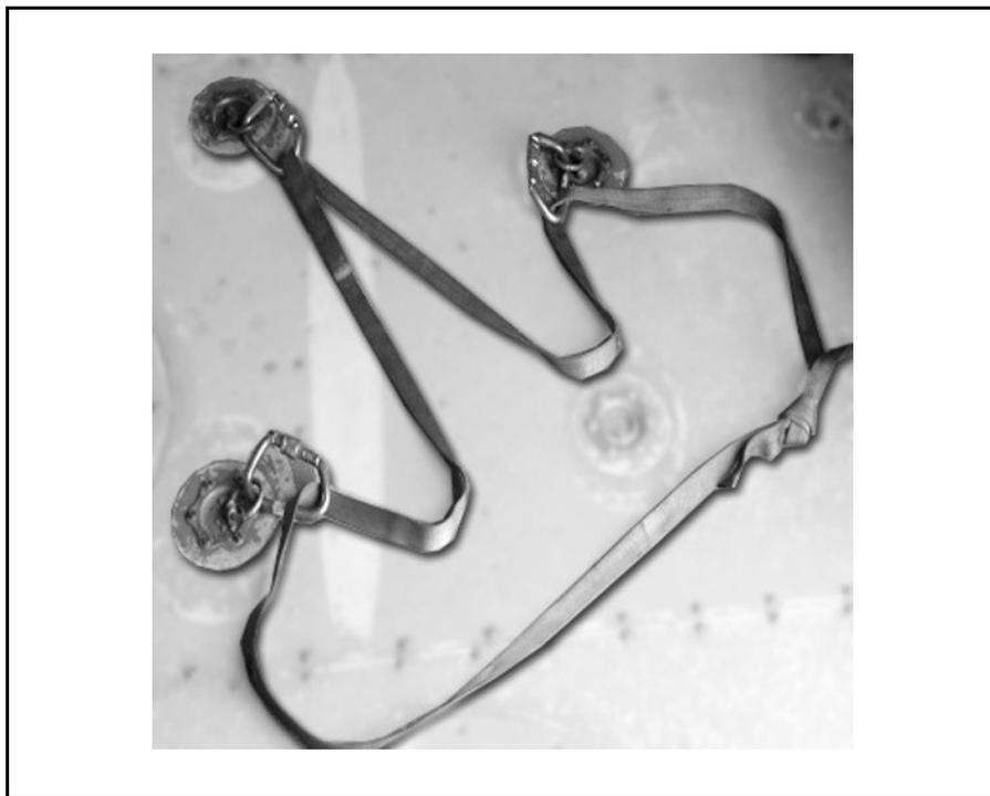
Figure 4-16. Cordelette Set-Up
