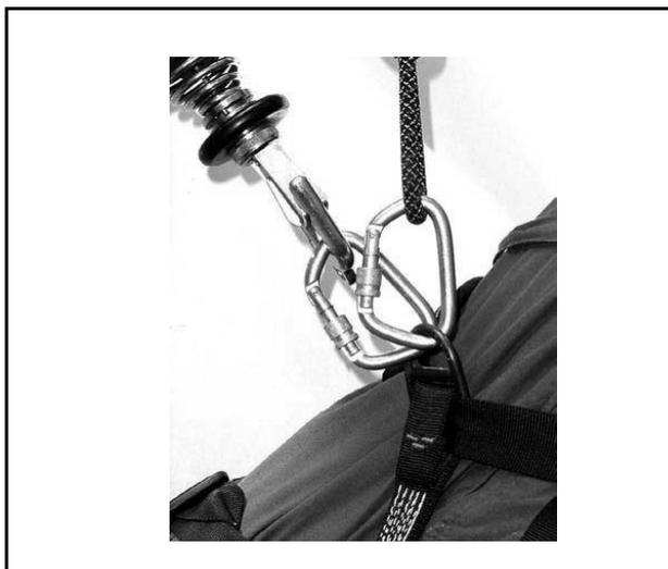
Figure 4-2. Single-Man Hoist to Rappel Harness
