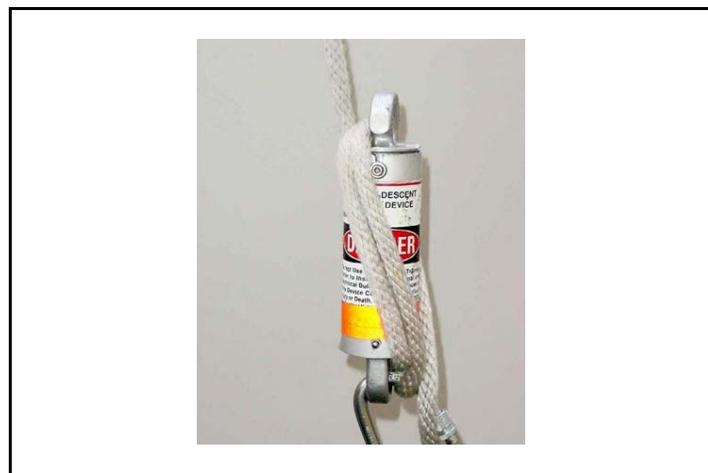
Figure 4-31. Descent Control Device Modified Lock-Off
