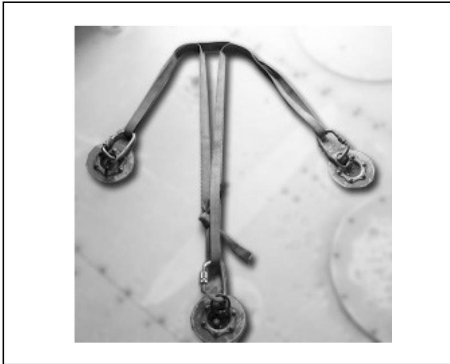
Figure 4-17. "V-Shapes" in Cordelette Deck Set-up
