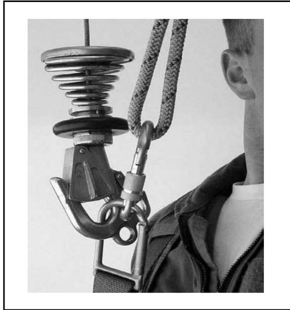
Figure 4-3. Single-Man Hoist to Integrated Torso Harness
