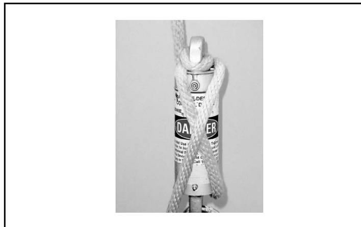
Figure 4-30. Descent Control Device Double Lock-Off
