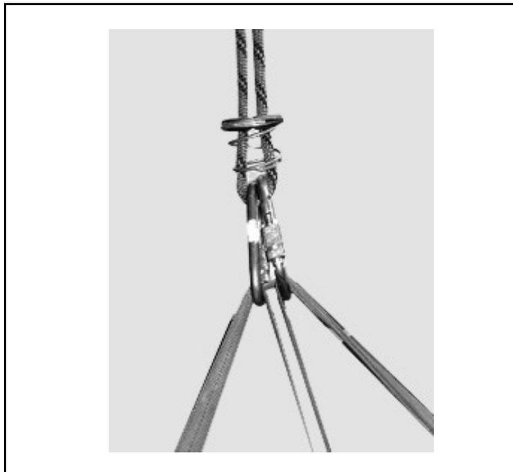
Figure 4-18. Belay Attachment to Cordelette Deck Set-Up
