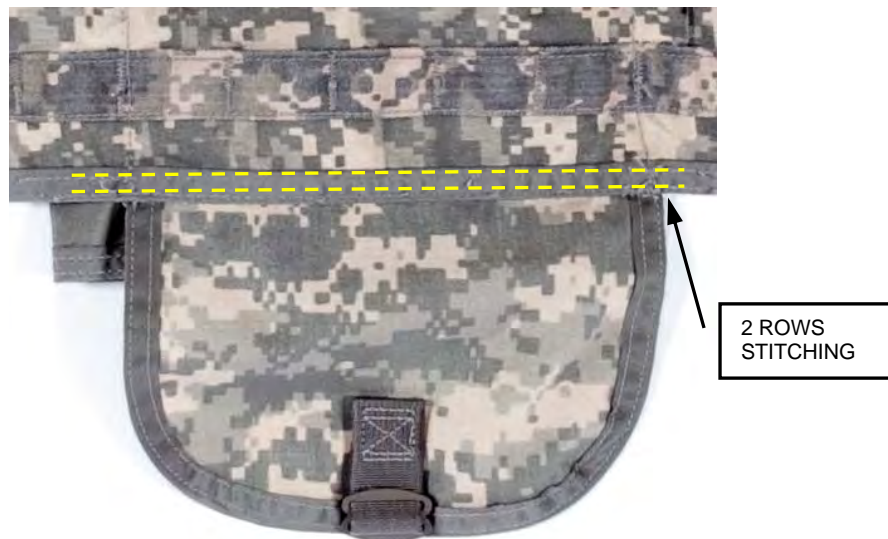
Figure 5. Sewing Plate Pocket Carrier Closed.
