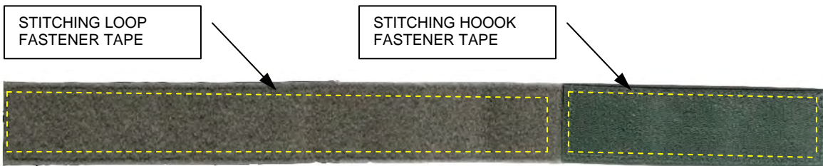
Figure 3. Vertical Attachment Strap Hook and Loop Fastener Tape Placement.
