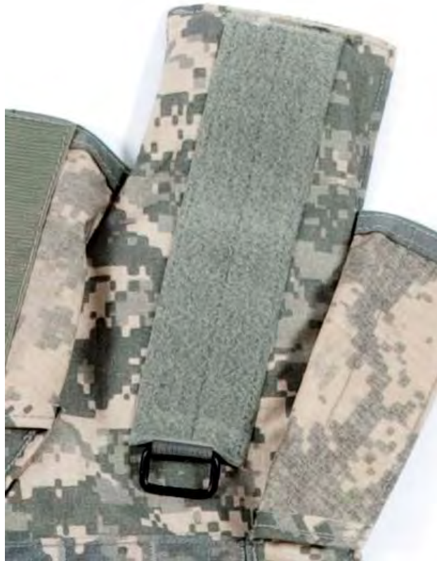
Figure 4. Damage to 2-Inch Loop Fastener on Left Outer Shoulder.
