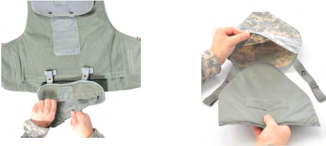
Figure 5. Removing Lower Back Protector and Groin Protector Soft Ballistic Inserts.
