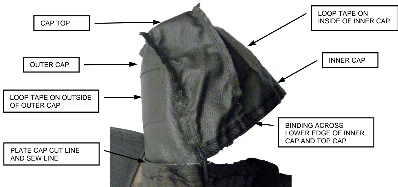
Figure 11. Side Plate Carrier Pocket Cap Construction (Shown Inverted).
