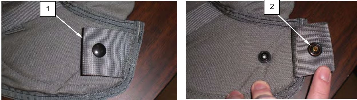
Figure 2. Repair Damage to 2-inch Webbing Attachment Straps.
