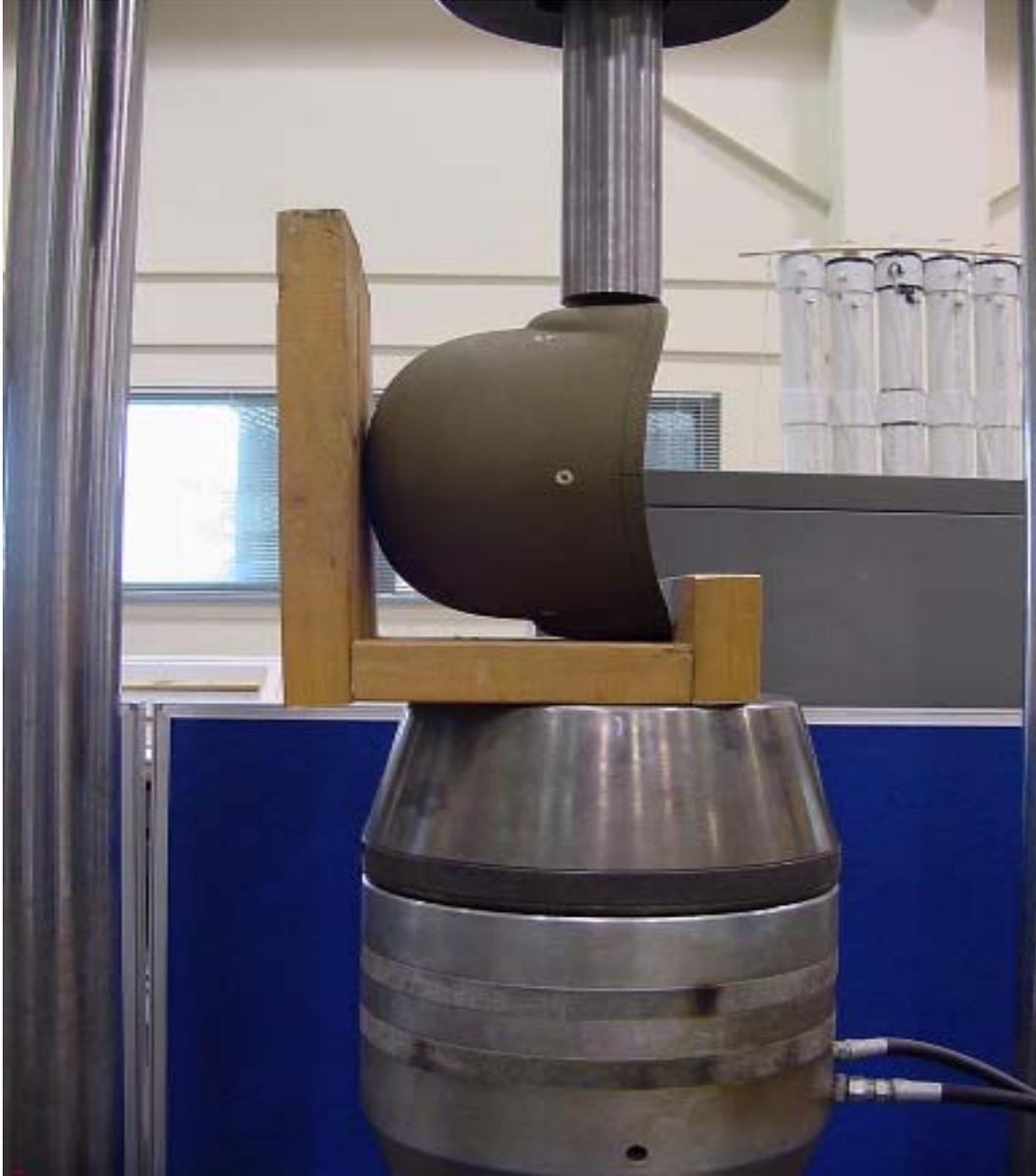
**FIGURE 5. Jig for side to side compression resistance.**
