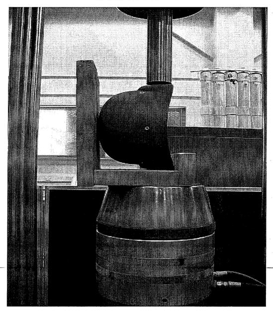
FIGURE 7. Jig for side to side compression resistance.
