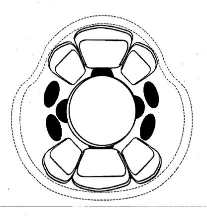
FIGURE 1. Standard helmet pad configuration.
