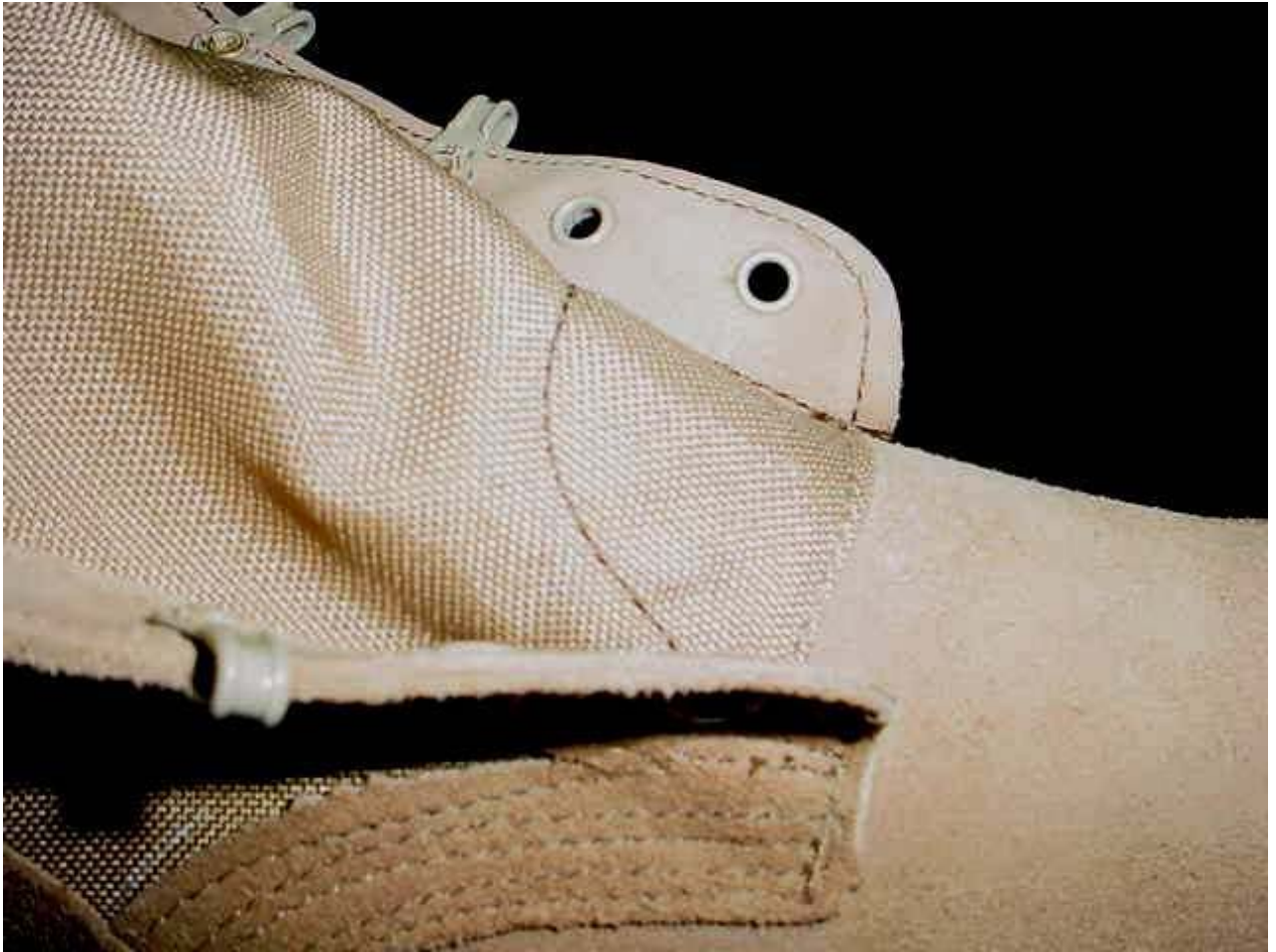
Figure 2b. Close up view of Vamp/Gusset seam (lateral view).
