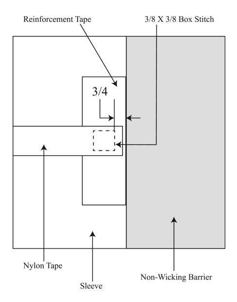
Figure 4. <u>Liner attachment tab assembly – View C.</u> Reinforcement tape and stitching detail.
