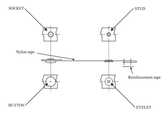
Figure 3. Liner attachment tab assembly - View B. Side view with snap detail.
