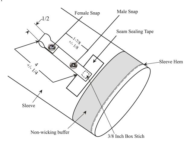
Figure 2. <u>Liner attachment tab assembly – View A</u>.
